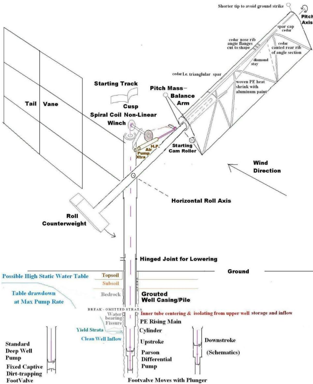
Fig 2 Schematic of the Flutterwell Pump, the Well-mounted FlutterWing Pump
